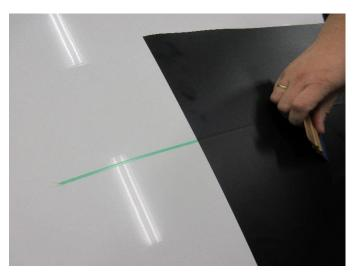
To remove air bubbles, press the film onto the Knifeless Tape again with your finger.
