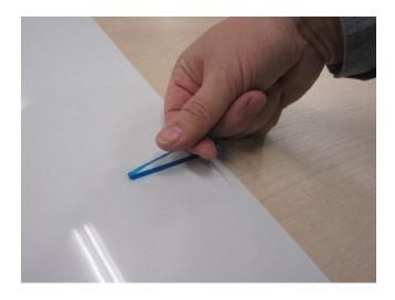
Press thumb firmly on folded edge, covering at least 1 cm tape.
