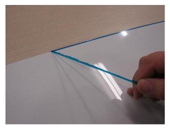
Heat the edges of the film and reapply the film edges with firm pressure.
