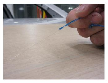
After cutting is finished, remove the excess film and the carrier tape from under the film. Assure that the carrier tape is completely removed without residuals.
