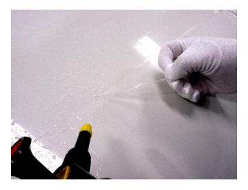
Apply the film edge to the substrate and re-press the film edge with pressure.
