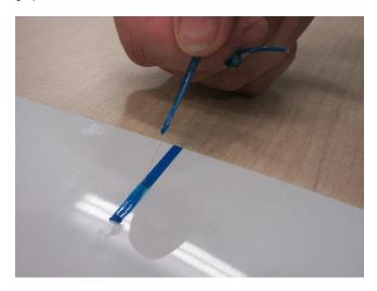
Fold the filament over the graphic. Press your thumb over both the filament and the graphic edge. Gently tug the filament to start cutting into the graphic, continuing to pull the line back and not upward.
