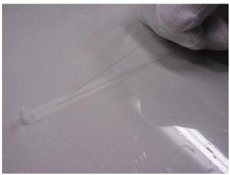
Tug the filament to start cutting into the film and the cover tape, continuing to pull the line back and not upward.
