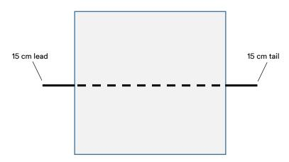
Begin with 15 cm of tape (before and after) where the graphic will be cut and lay down Knifeless Tape. Apply the film with pressure over the Knifeless Tape, leaving the lead and tail tape visible.
