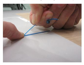
Firmly grasp the end of the tape with your thumb and index finger positioning your two thumbs close together to start the filament. Gently pull the line to tear the carrier tape and expose the filament. Pull the line back and not upward, stopping before the edge of the graphic.
