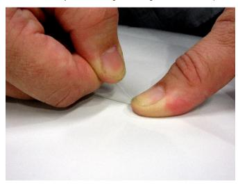
Firmly grasp the end of the tape with your thumb and index finger, positioning your two thumbs close together to start the filament. Gently pull the line to tear the carrier tape and expose the filament. Pull the filament back and not upward. Tack end of filament to vehicle until ready to cut film.
